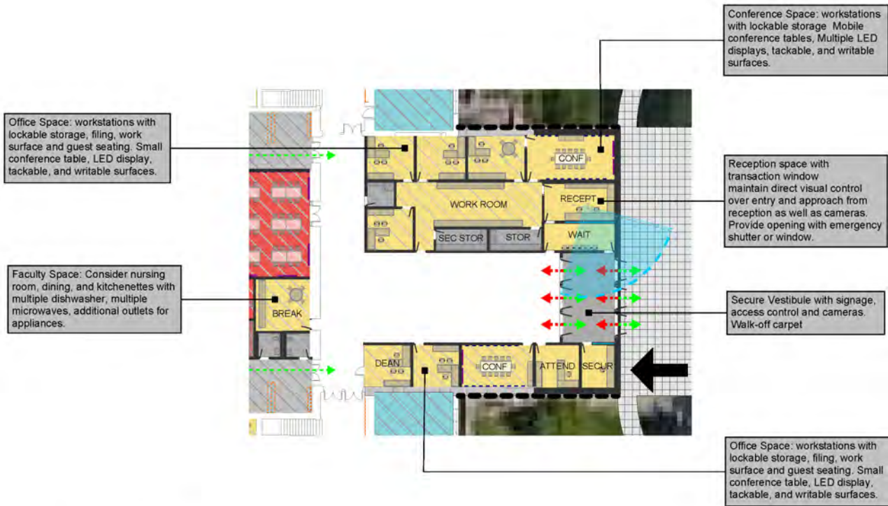
First Floor Remodeling - Center Section (Administration) Scale: 1"=20'-0"
